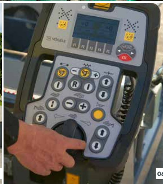
04 PaveDock Assistant communication system for optimum material feed 05 Large material hopper with a capacity of 13 tonnes 06 ErgoPlus 3 screed operator's console with SmartWheel for convenient screed width control
