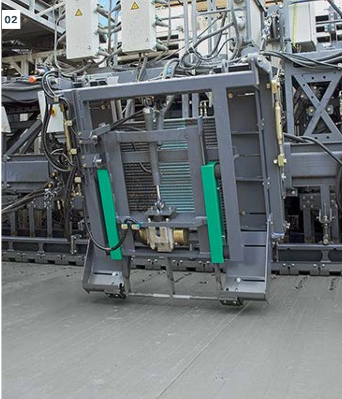
01 Distribution of the dowel bars by means of an intelligently designed chain system.
