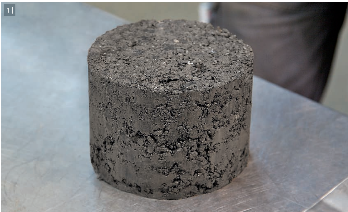
1 | Material treated with foamed bitumen is distinctive for its optimal strength and bearing capacity.
